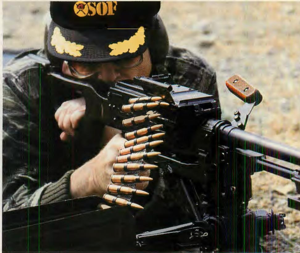
sheet-metal stampings in other areas, especially the top cover and feed mechanism. This is 5.5 pounds less than the M60. Its excellent lightweight tripod (with aluminum legs) tips the scales at only 10.4 pounds. Overall length of this weapon is 47.7 inches. The four-groove, non-fluted
